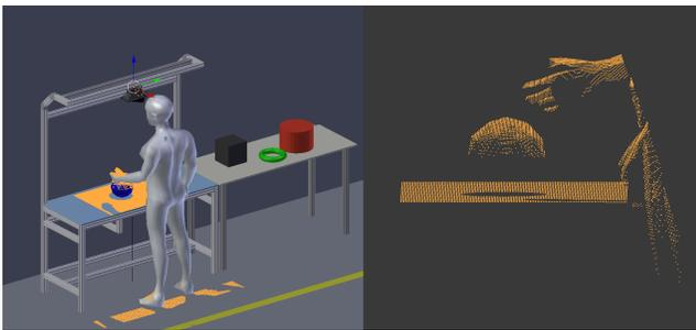
Fig. 5. Example of virtual commissioning of an image-based component.
